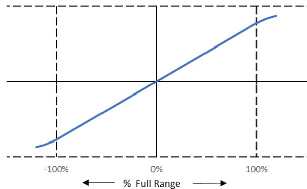
Figure 4 – The output from an LVDT signal conditioner is a linear DC signal that can be accepted by most control systems and meters.
