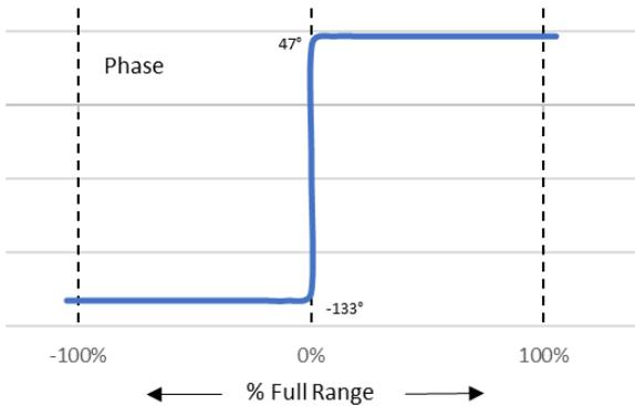
Figure 3 – The phase of the LVDT output abruptly shifts  $180^\circ$  as the core travels through the null point.
