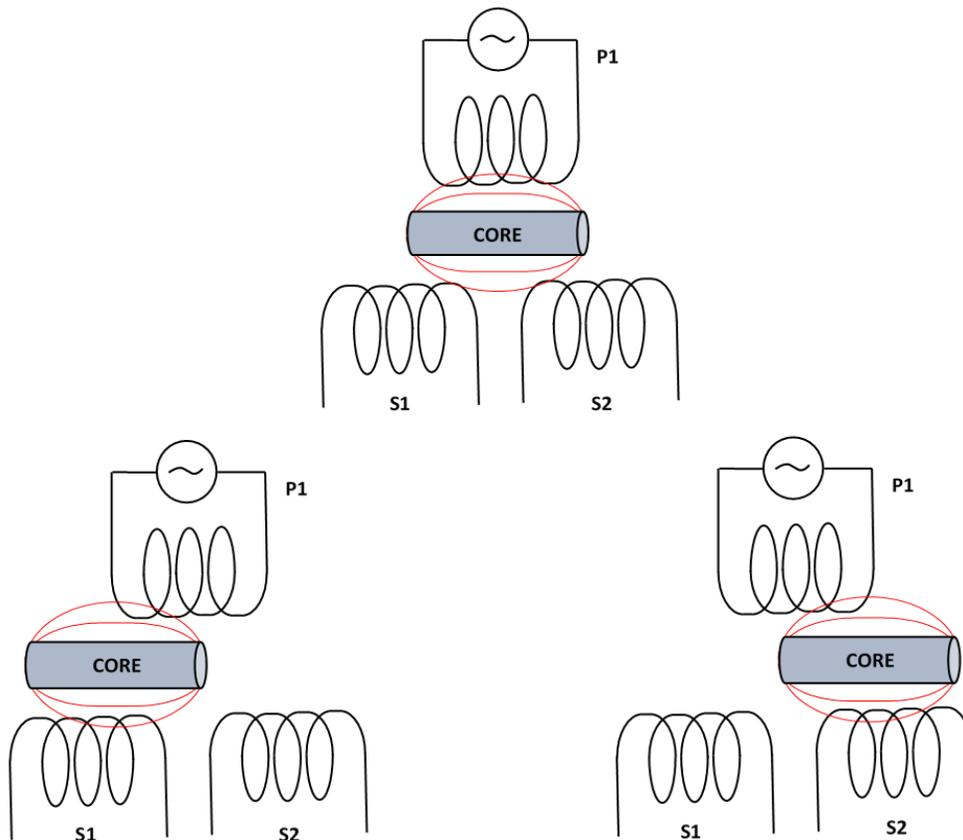
Figure 1 – As the core moves within the LVDT, it further engages with the secondary winding it is entering and disengages from the winding opposite. The difference between *S1* and *S2* gives an electrical signal proportional to the core position.
