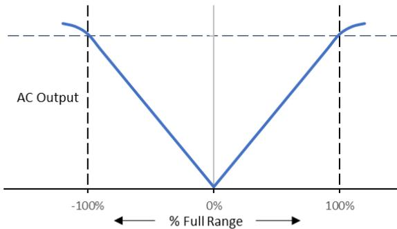
Figure 2 – The AC output increases as the core moves away from the null point in either direction.
